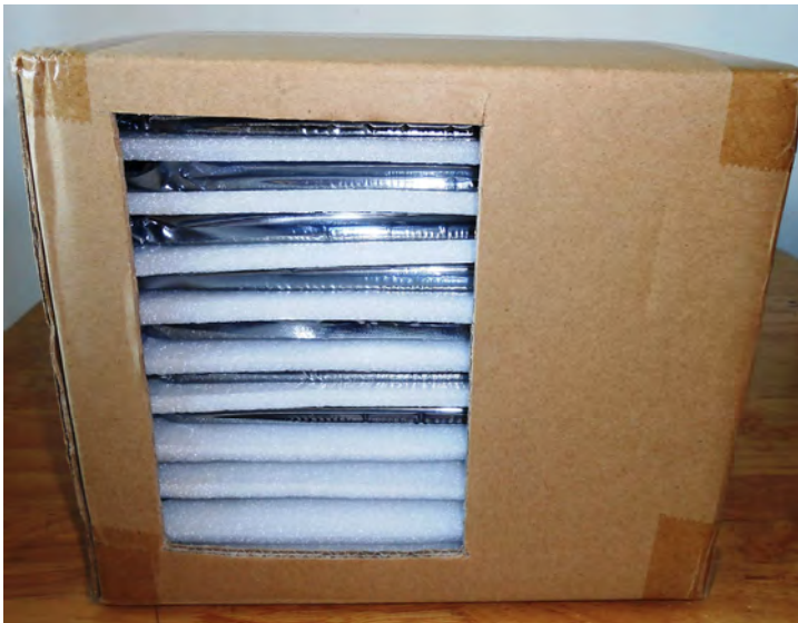
Place Foam Sheets and Trays into Box
